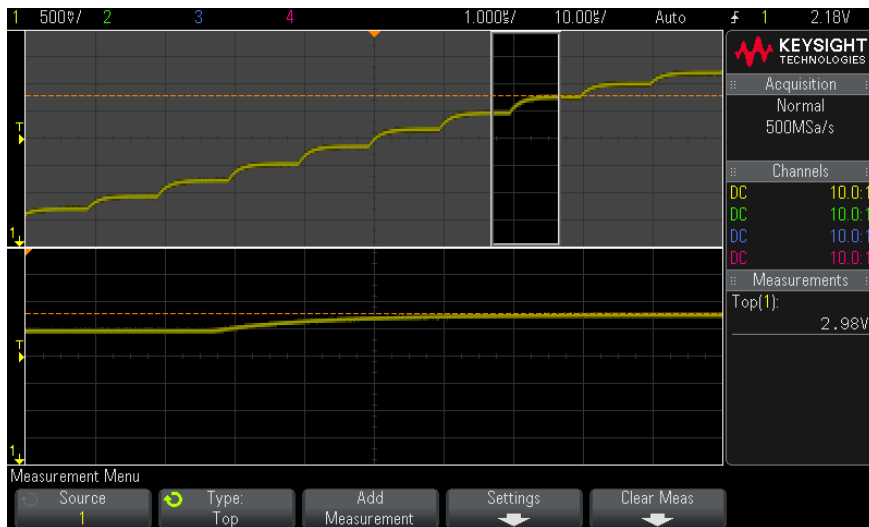
Figure 33 Isolating area for Top measurement
